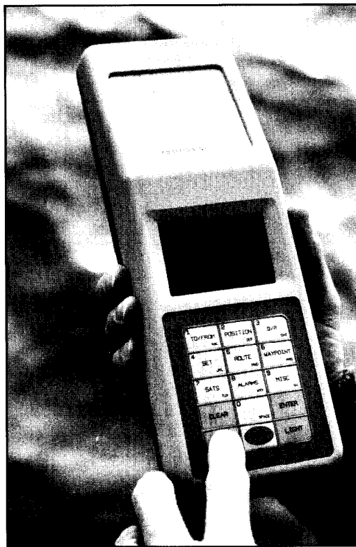
Figure A. Gypsy hand held receiver.
